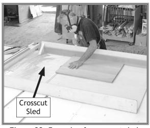
Figure 82. Example of a crosscut sled.
